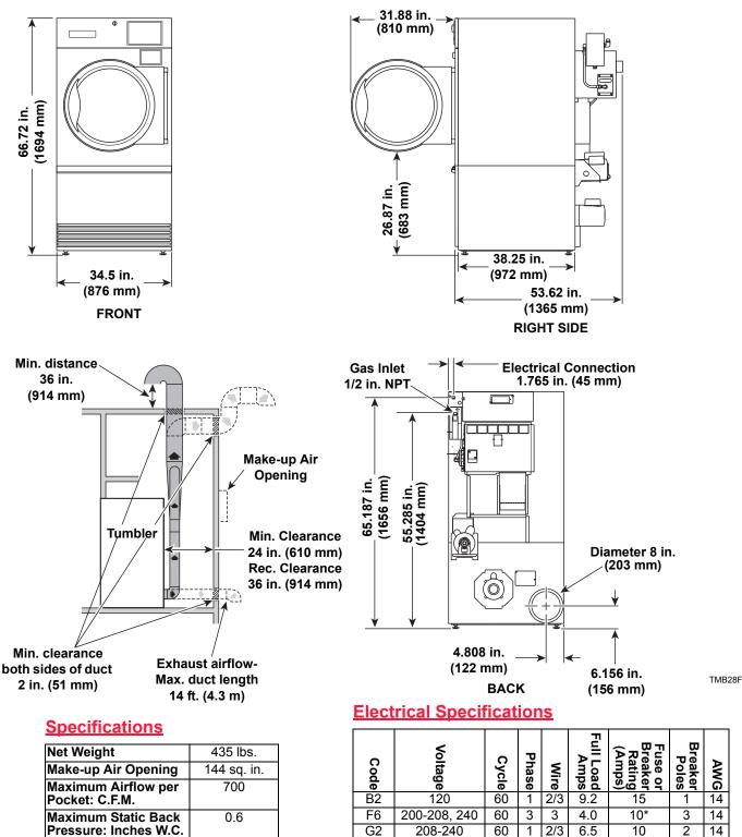
\* 3 Phase machines should not have fuses, breakers only.
